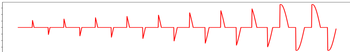
Soft start with ON/OFF, Burst, Distributed full cycle and Advanced full cycle firing modes
